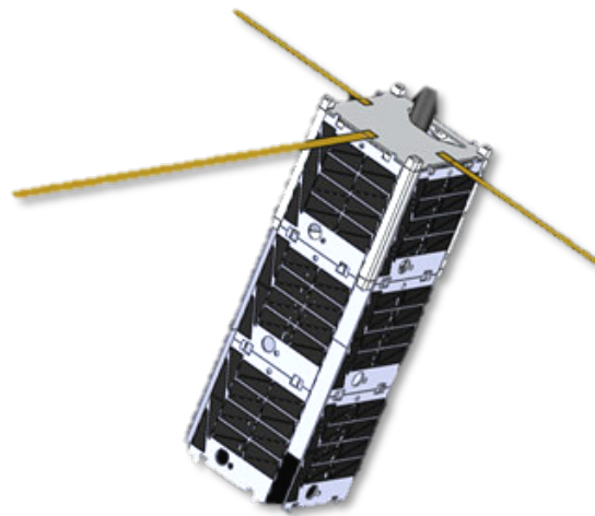
Figure 2 - Lambdasat picosatellite (Courtesy Lambda Team)
