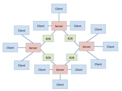
Figure 6. Distributed Server Simple Partial Mesh Configuration
